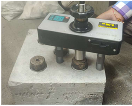
Fig. 8 –Pull-off test set up
