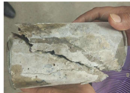
Fig. 7 – Test specimen after slant shear test
